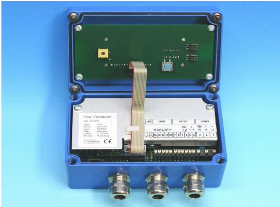
Abb. 2: LCD display connection with cover open
